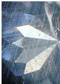
[Rutile needles (silk) aligned in three directions in unheated corundum]
