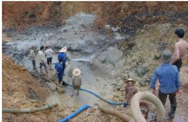
*[Tan Huong, Vietnam, ruby and spinel mine. Back hoes remove about six feet of soil then high pressure water is used to loosen the old buried stream bed so the miners can use screens and sluices: Image courtesy of [www.gemsfromearth.com](http://www.gemsfromearth.com)]*
